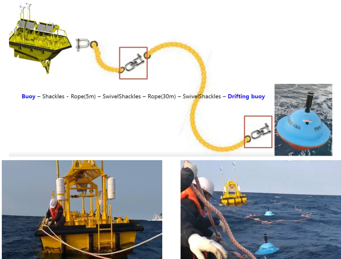
Fig. 2. Design of experiment for analyzing the characteristics of wave observed from ocean data buoy and drifting buoy.
