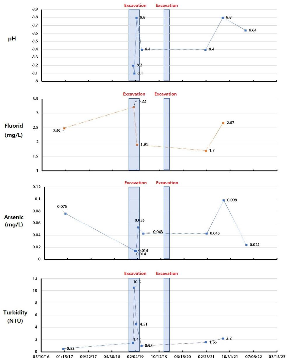
Fig. 4. Change of GW1 groundwater quality in relation to tunnel excavation.
