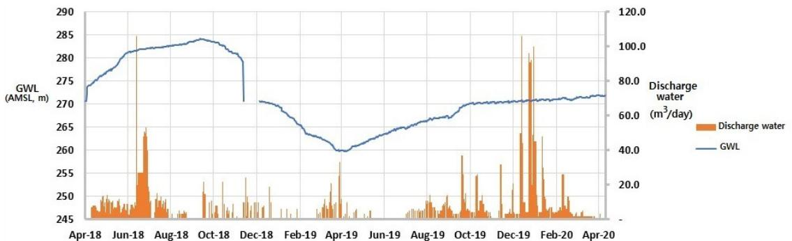
Fig. 3. Relationship between tunnel discharge and groundwater level (GWL) of the GW1 well.
