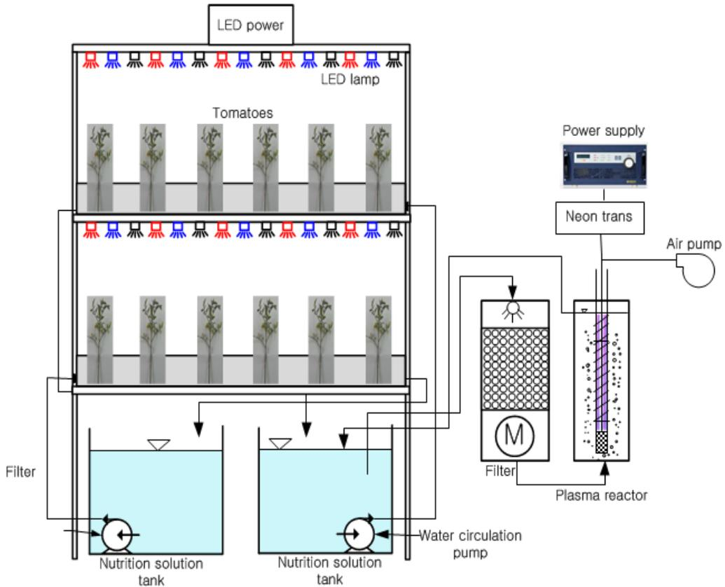
Fig. 1. Schematic diagram of nutriculture system and plasma system.
