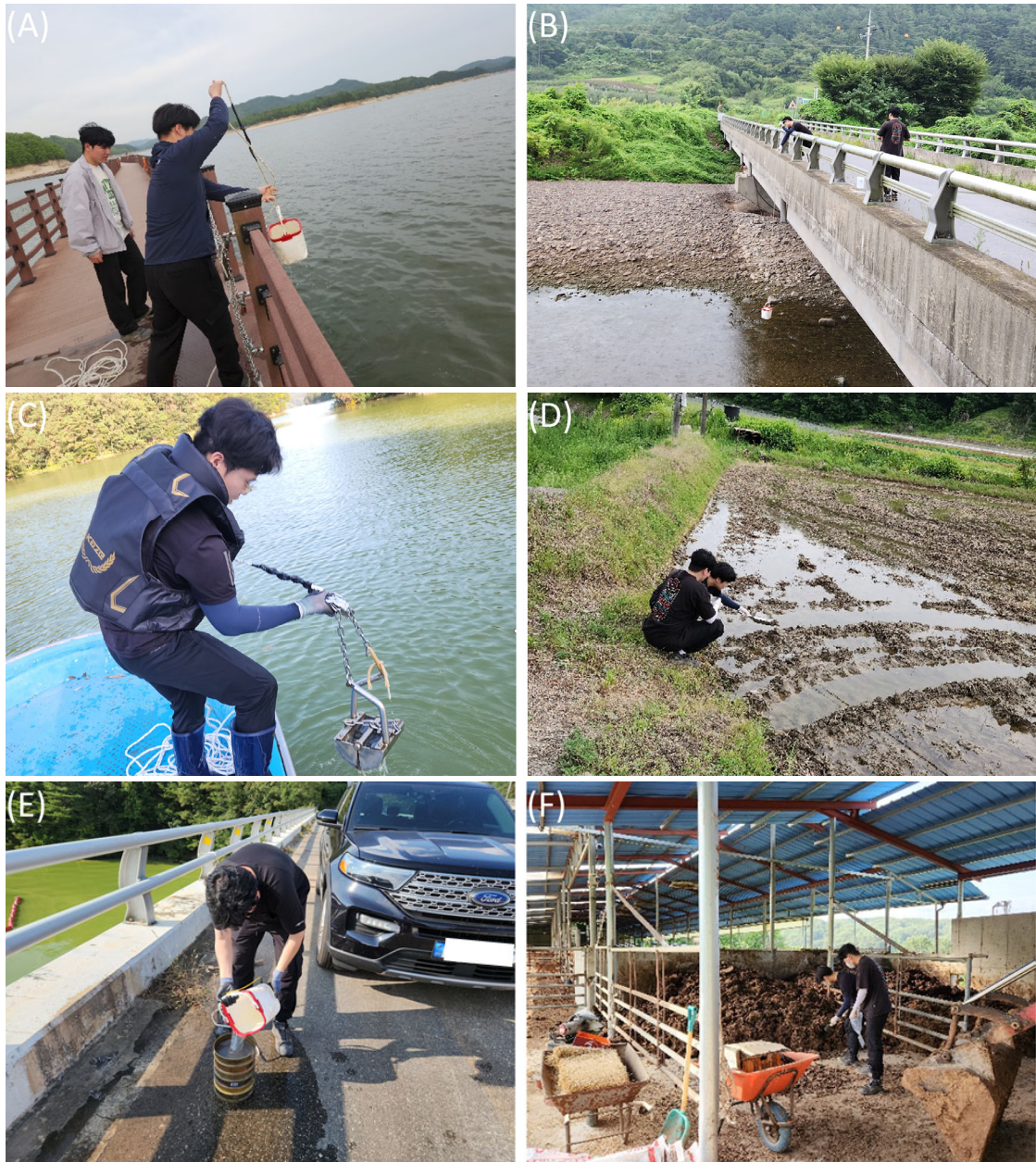
Fig. 2. Field sampling of water, sediment, soil, algal bloom, and cattle manure. (A) Surface water sampling at a reservoir site, (B) Water sampling at a tributary bridge, (C) Sediment sampling using a grab sampler, (D) Soil sampling in an adjacent agricultural field, (E) Collection of algal bloom, (F) Cattle manure sampling.
