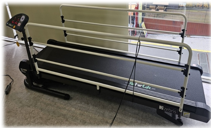
Fig. 1. Zebris pressure-sensitive treadmill system used in this study.
