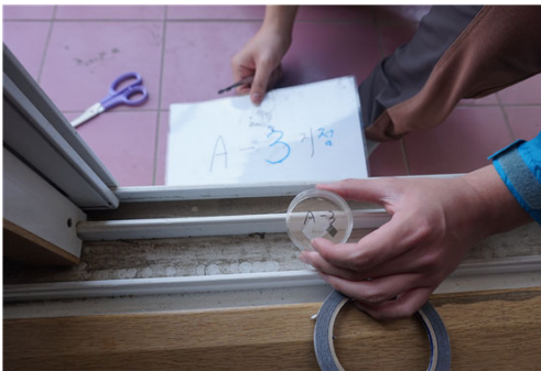
e) deposited dust collection and SEM/EDS analysis
