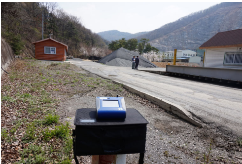
c) concentration measurement by light scattering method
